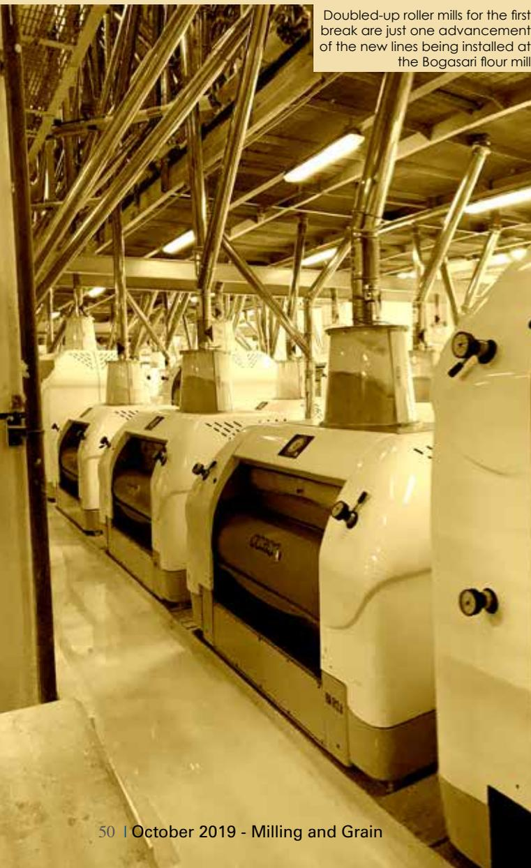
Doubled-up roller mills for the first break are just one advancement of the new lines being installed at the Bogasari flour mill
