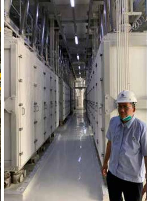
Pansifiers were the first to be replaced in a two-step operation that did not hinder the output of the three lines being upgraded
